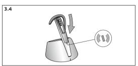
3.4 Place headset in charge cradle and charge for a minimum of 30 min. before use. A full charge takes about 2 hours. Visual indicator on headset will flash green while headset is charging, and light steady green when fully charged. The same procedure is to be followed when using the travel charger.
